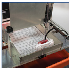
Pneumatic Air Cylinder Inserts the Patient Doc
