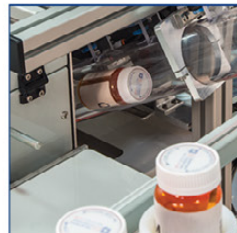
Maximum of 4 Bottles can be Deposited at a Time
