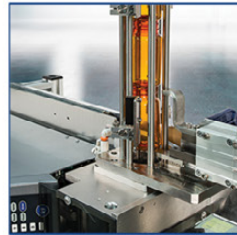
Labels 900 Bottles Per Hr Speeds of 4" to 8" Per Sec
